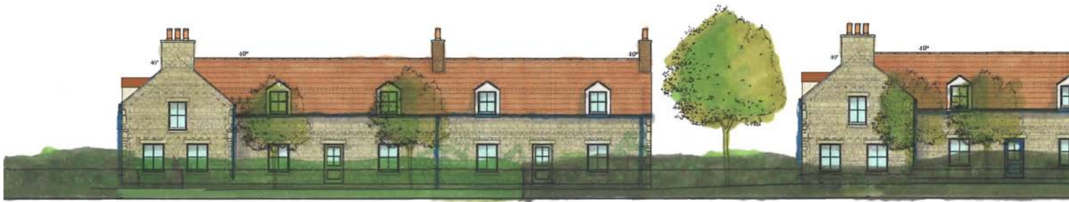
1. A street elevation showing the proposed frontage to south side of Winston Road. The houses are 1.5 storey with gables facing onto the street at each end. The frontage to Winston Road has been designed as a single composition to achieve a calm and ordered elevation.
