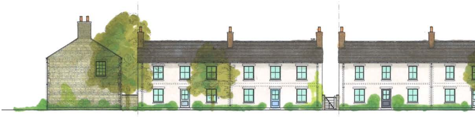
2. View of terrace of cottages facing onto the linear green space. The materials are a rendered wall finish with slate roof tiles.
