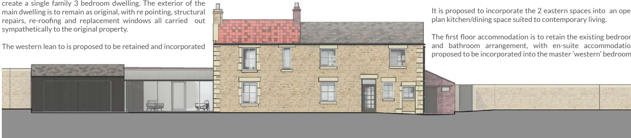
Fig 6.2 - Croft House - Proposed Southern Elevation
